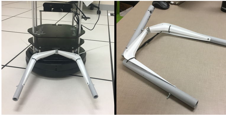
Figure 1: U-Guide attachment used on the kicker robot to capture the red soccer ball.
