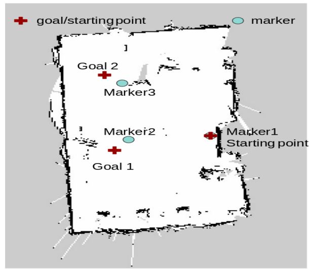
Figure 3 Markers layout and the navigation goals design on RVIZ map: the turtlebot navigates towards the first goal and the second goal.
