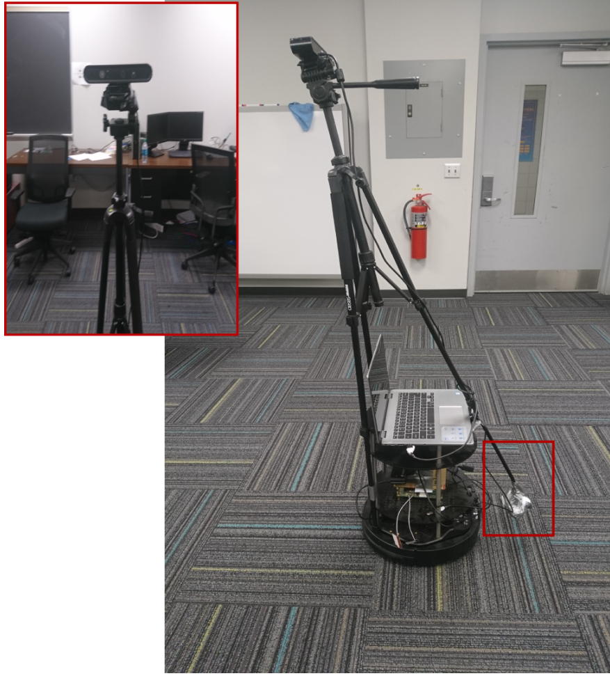
Figure 1 Figure showing the turtlebot setup. The setup contains the base of the turtlebot, the laptop on top, the tripod holding a depth camera for human detection, a depth camera – not visible– for navigation, and a balancing weight fixed to one end of the tripod.
