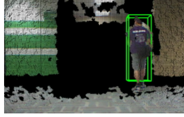
Figure 4: Example of human detection with RGB-D sensor.
