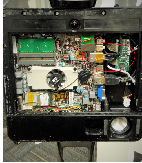
Figure 2: Beam's screen has been taken off to access the Ethernet port inside its Head. The circled areas highlights the Ethernet port.
