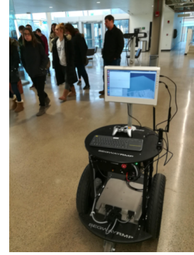
Fig. 1. Segway-based mobile robot platform used in this research.
