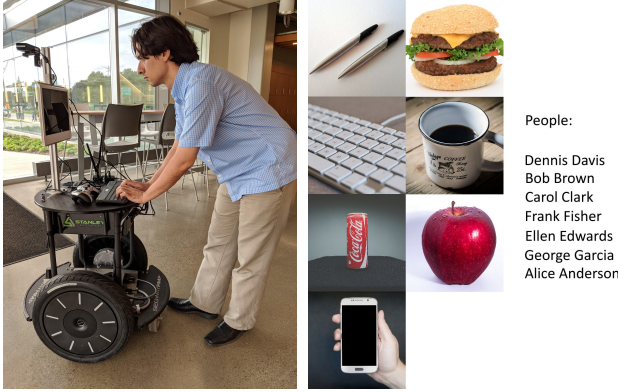
Fig. 7. Left : Segway RMP110 used in the experiment. Right : List of the items and recipients that robot participants used to ask for delivery. Two items and two people were unknown to the robot.
