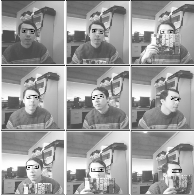
Figure 10: (B) Sample frames of detected and tracked eyes from a video sequence captured by an active web-cam. From top-left to bottom-right: frame 1, 73, 145, 250, 360, 425, 490, 515 and 540.
