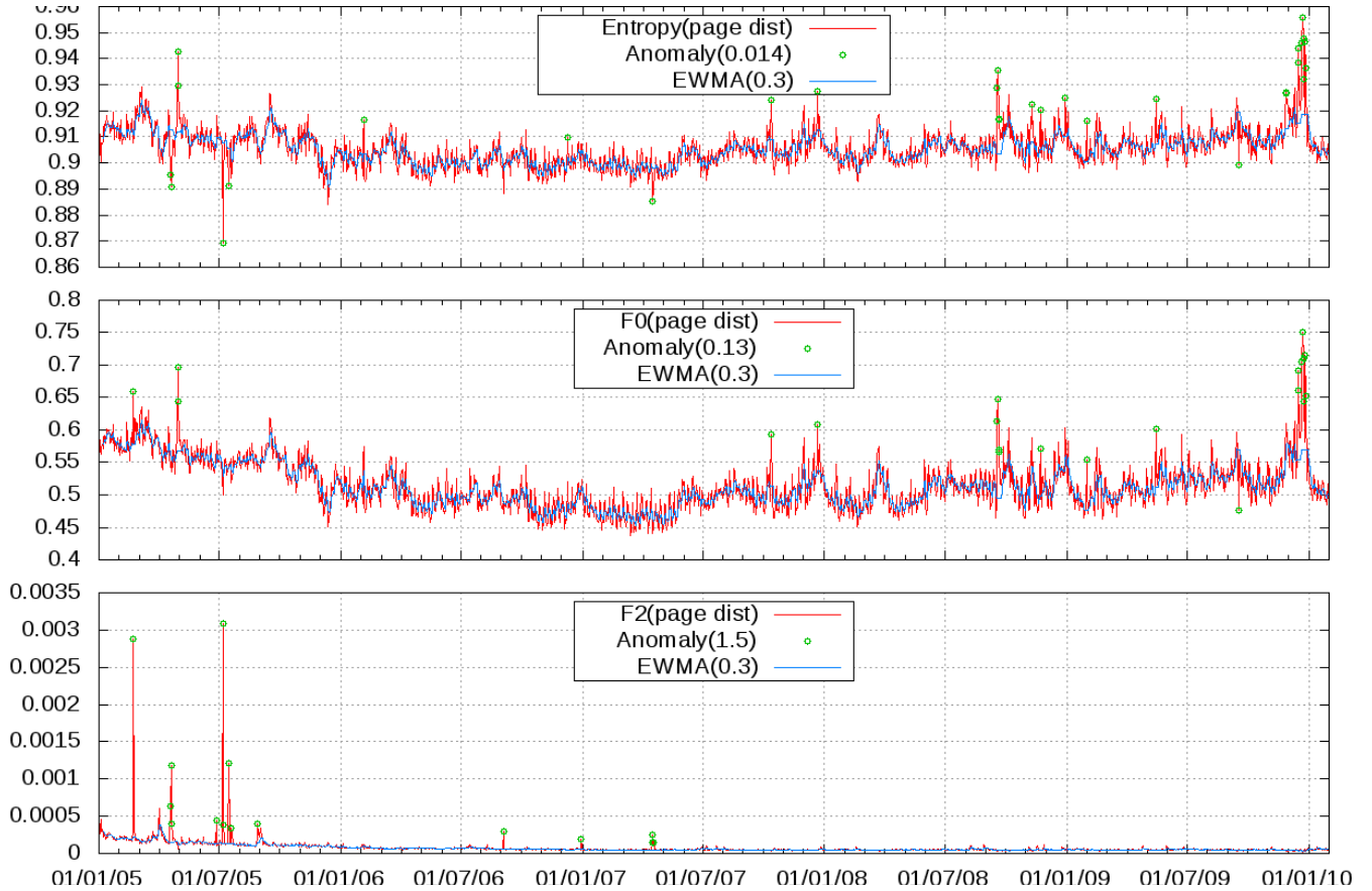
Fig. 5. Anomaly detection with the page distribution timeseries. Y-axis is metric value. [Best viewed in color.]
