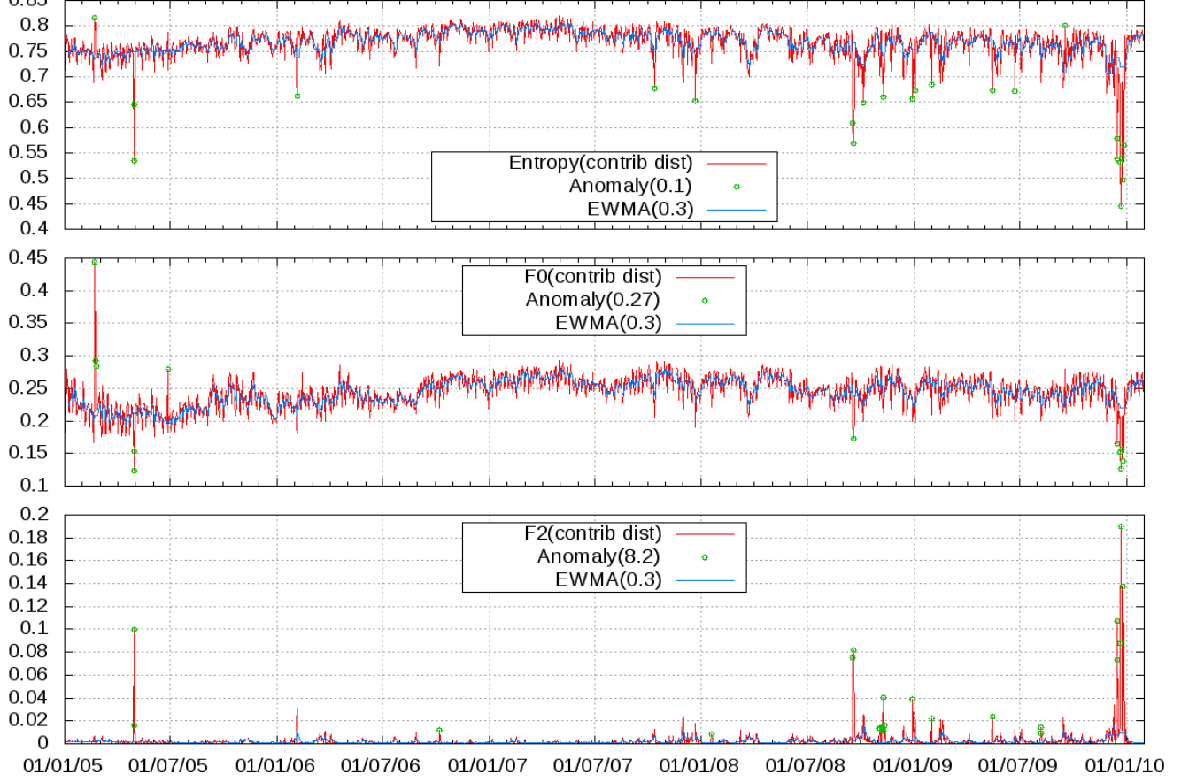
Fig. 6. Anomaly detection with the contributor distribution timeseries. Y-axis is metric value. [Best viewed in color.]
