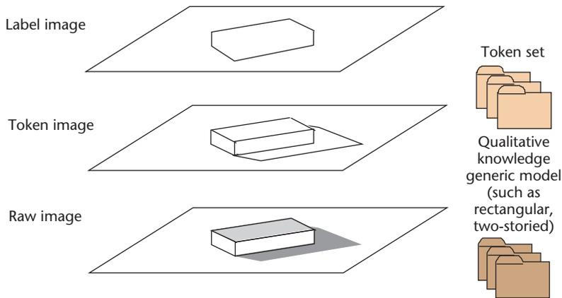
**Figure 5. Illustration of building detection.** Given a raw image, we apply a line-finding algorithm to the raw image to obtain a line token image. This is followed by line grouping to detect buildings.
