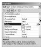
Manipulating the Anchor property of a control.
