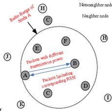
Figure 2. Operation of the transmission power control
