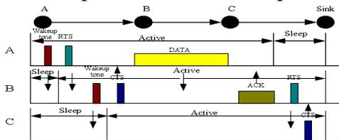
Figure 3. Operation of the duty-cycle scheduling
