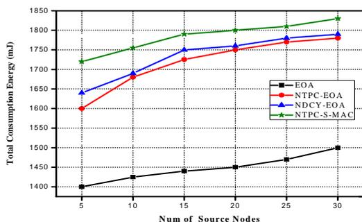
Fig.9. Total energy consumption according to the number of source nodes
