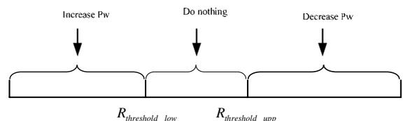
Figure.3. Adjusting transmission power level
