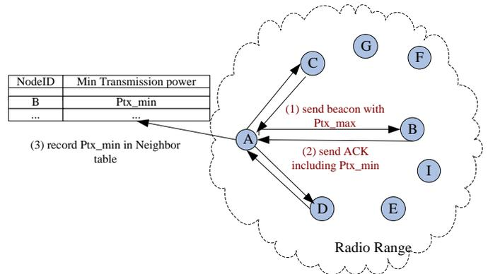
Figure.2. Operation of transmission power control
