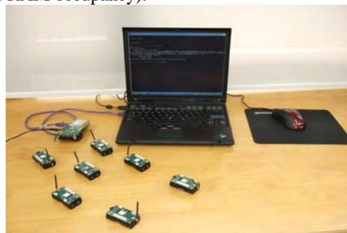
Figure.6. MicaZ mote Test-platform
