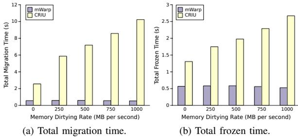
Fig. 6: Varying dirtying rate on live container migration.
