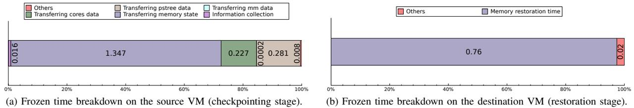
Fig. 2: Breakdown of frozen time at each stage of live container migration.
