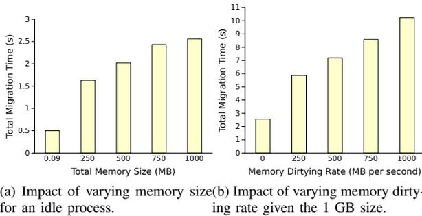
Fig. 1: Impact on total migration time by varying memory size and varying memory dirtying rate.
