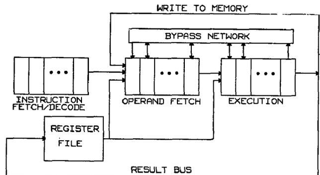
Figure 7. Example of a linear pipeline implementation.
