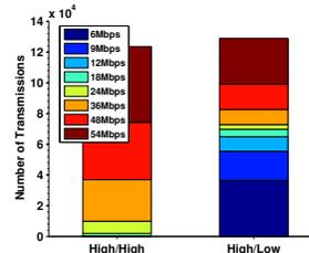
Figure 1: The number of packets transmitted at each data rate of an 802.11g WLAN carrying two video streams. The High/High case represents the setup where both video streams are over a high data rate link and the High/Low case represents the setup where one stream is over a high data rate link and the other is over a low data rate link.
