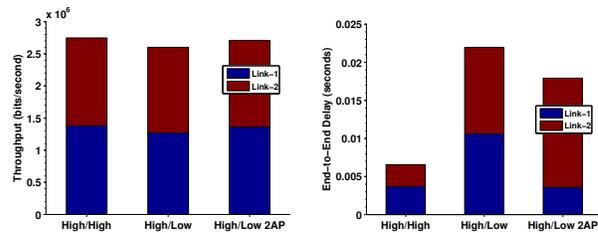
**Figure 3: Using Multiple APs prevents performance degradation of high data rate links.**
