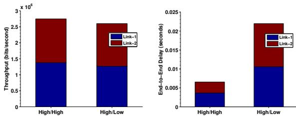
**Figure 2: Slight decrease in throughput due to the rate anomaly problem. However, because the low data rate link transmits for a much longer duration, the end-to-end delay is increased significantly for both links.**
