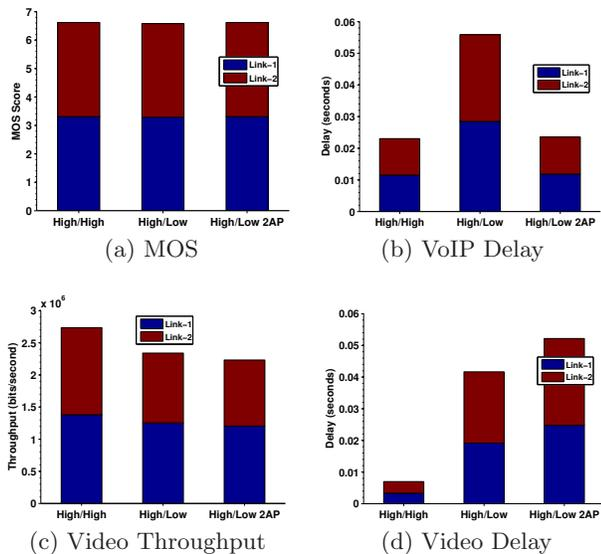
Figure 4: Using Multiple APs prevents performance degradation of high data rate links.
