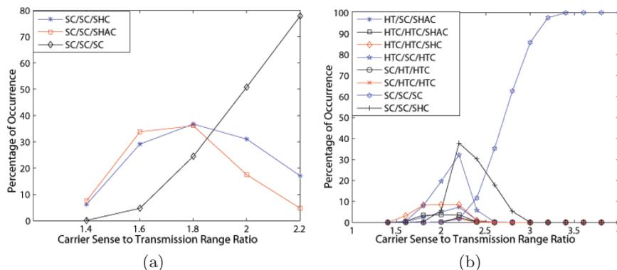
**Fig. 3.** Occurrences of Different Types of Chains. (a) shows the occurrence probability of 3-hop chains.(b) shows the occurrence probability of 4-hop chains.
