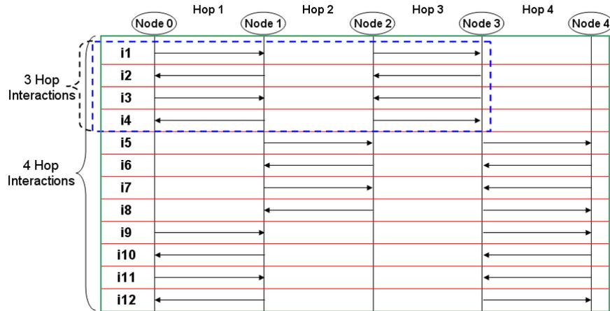
**Fig. 2.** All the interactions in a three and four hop chain. Each row shows the interaction between two specific links in specific directions.
