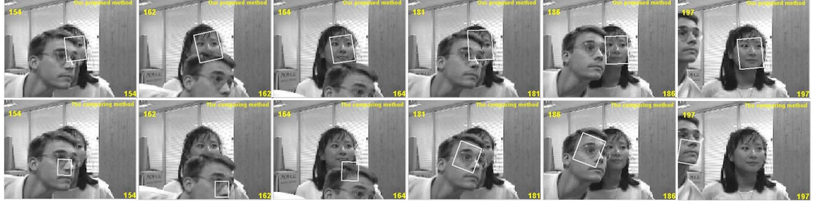
Figure 5. Tracking results of IRSL (row 1) and CTMU (row 2) over representative frames in the scenario of a severe occlusion.
